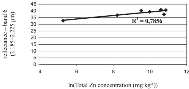
Figure 2. Relationship between reflectance in spectral range 2.185–2.225 μm and zinc concentrations in smelter waste barren of vegetation.
